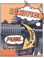
Once the turbine is clear, it slows down to 14% speed or 504 RPM. Fuel starts to flow and IGNITION IS ACTIVATED!
