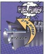
This initiates the turbine rotor to rotate at 27% speed or 972 RPM. This spinning causes air to move through the turbine and flush out any residual fuel fumes.
